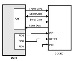
Figure 8-5 DBRI and CODEC Interface
