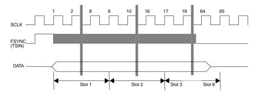
Figure 8-8 Frame Timing
