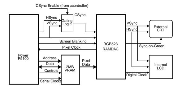
Figure 11-2 Display Interface Timing
