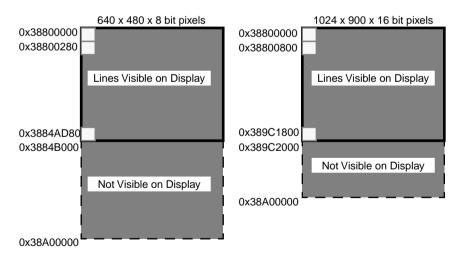
Figure 11-4 Frame Buffer Addressing
