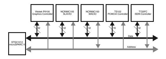
Figure 1-4 SBus Connected Devices
