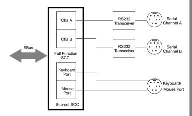
Figure 4-1 Serial Interface Architecture
