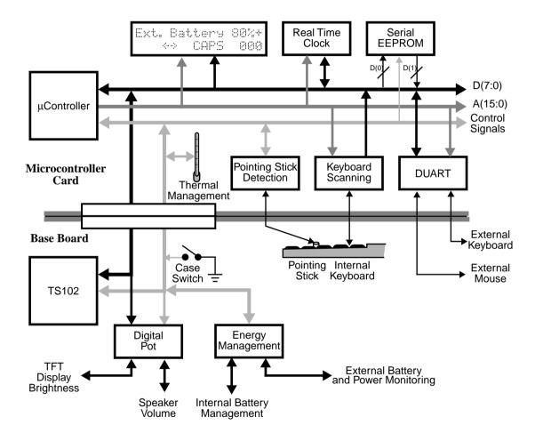
Figure 12-1 Microcontroller Subsystem Architecture
