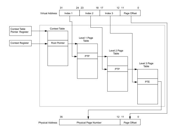
Figure 2-5 A Three Level Table Walk In Memory
