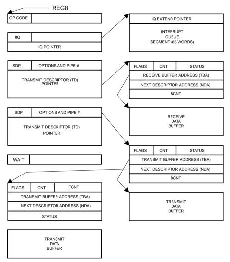
Figure 8-4 DBRI Data Structures
