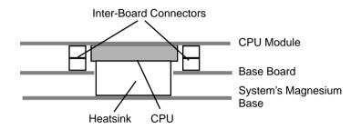
Figure 1-1 CPU Heat Dissipation
