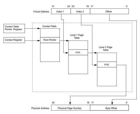
Figure 2-6 A Two Level TableWalk In Memory
