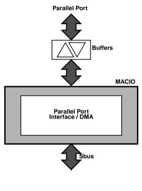
Figure 10-1 Parallel Port Architecture
